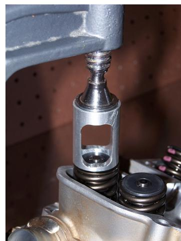
Figure 2. Proper Valve Tool positioning
